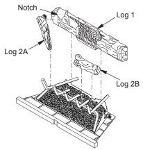
Figure 29 - Installing Logs 1, 2A and 2B
